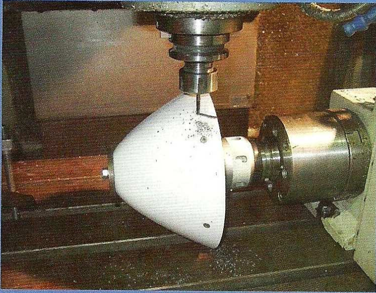
New nose cone/spinner, drilled for fixing to motor
