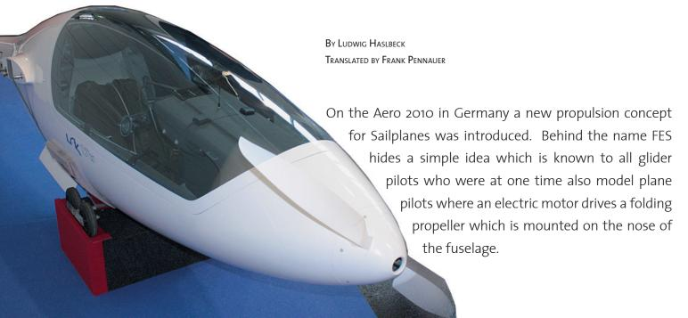
his propeller folds itself smoothly against the fuselage during soaring flight, without creating any appreciable additional drag and it opens whenever engine power is applied. It is not surprising that the developers of this concept, Luka Znidarsic and his son Matija are not only glider pilots but also avid model plane builders.
